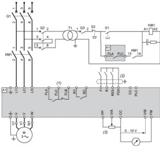
A1: ATV 212 drive KM1: Contactor Q1: Circuit breaker
