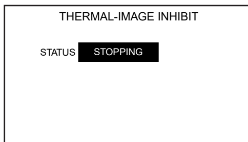
Figure 53 – Thermal-Image Inhibit Stopping Screen
