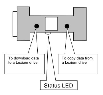
After the module is connected to the X6 connector, the status LED is on.
