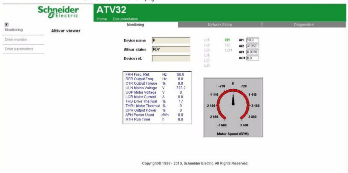
The state indicated in the "Altivar State" field corresponds to the display on the drive integrated display terminal. A delay may sometimes be noticed between the displays on the Web server and the display terminal, depending on the performance of the computer used to display the pages using a Web browser and the communication system performance.
