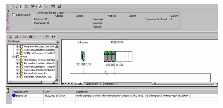
The VW3 A3 616 module is identified with the symbol: Generic Module. This identifier will be used later with tools such the Class Instance editor.
