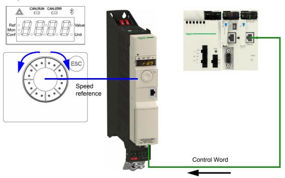
The drive is controlled from the communication (EtherNet) but the reference is adjusted on the local HMI. The control word comes from the controller and is written according to CiA402 profile.
