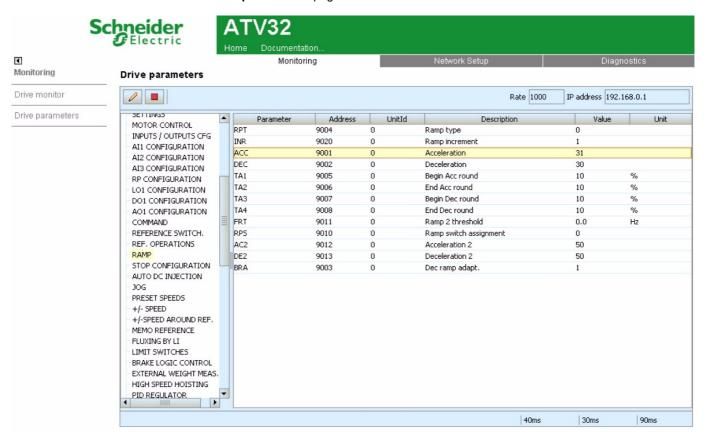
This page is used to display the drive parameters and to modify their values.
