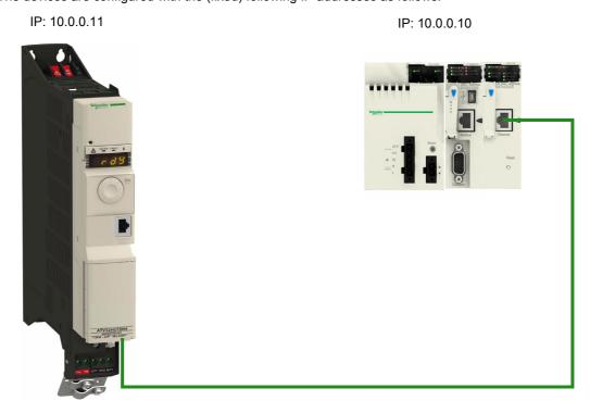
The ATV32 will be controlled through the option communication scanner by means of the I/O scanning service.
