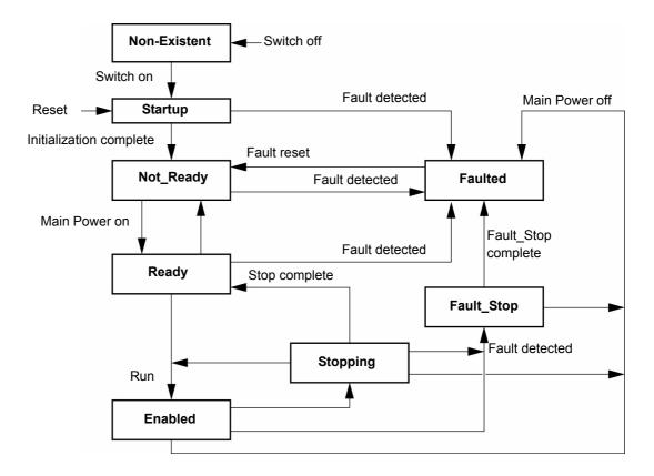
The Servo 3 drive state machine shall be supported as well. This state machine is already defined by D-SW.
