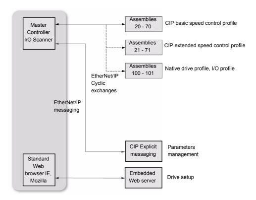
The Altivar 32, equipped with the VW3 A3 616, is compliant with the ODVA drive profile. It supports the 3 following profiles:
