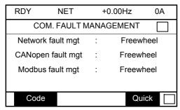
The values of the [Network fault mgt] ( $\mathcal{L} L$ ) parameter, which trigger a drive detected fault [Com. network] ( $\mathcal{L} \mathcal{D} \mathcal{F}$ ), are:
