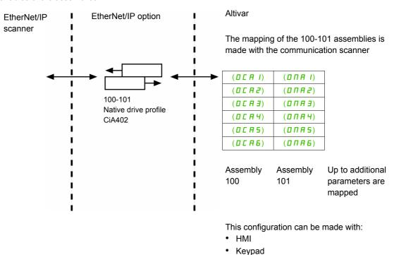
The size of the assembly (100, 101) is fixed and is equal to 6 words.
