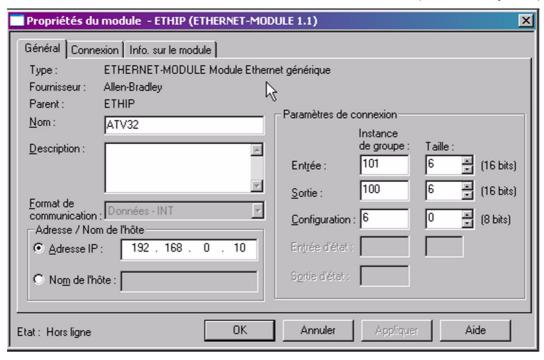
Once configured, the data objects are automatically updated and linked with the implicit exchanges mechanism:
