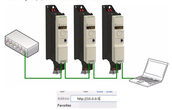
First connect the PLC to the ATV32 by typing http:// followed by the ATV32 IP address. You will be asked to first enter a User Name and a password.
