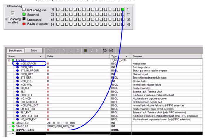
The exchanges can be stopped by setting to 1 the pending bit in the array %QW0.1.0.0 (in the example).
