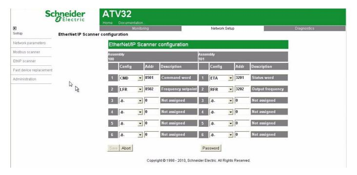
A dropdown menu is used to modify the assignment of each of the periodic variables.
