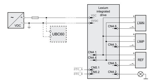
The UBC60 braking resistor controller is available as an accessory, refer to the chapter Accessories and Spare Parts *(see page 225).*
