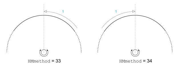
1 Movement to index pulse at velocity HMn\_out
