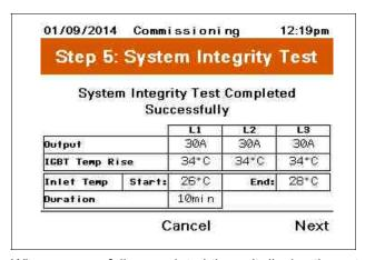
When successfully completed the unit display the output current values per phase, IGBT temperature rise during the test period. The inlet air temperature at the start and end of the test, ant the duration time of the test.
