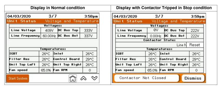
Contactor State: Provide information on why the contactor is tripped.
