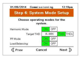
When Harmonic mode is selected, a Target THDi or THDv can be set. Leaving the Target at zero will result in the unit doing the best possible correction.
