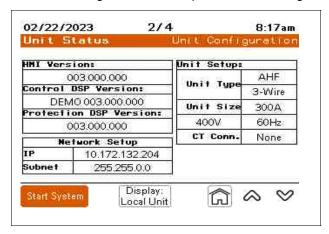
HMI Version: Displays the HMI software version that is loaded on the HMI.
