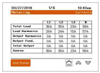
Total Load: Total load current in amperes RMS.
