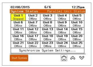
The Parallel Unit Status provides general operating condition of each unit in the parallel system.
