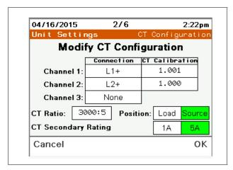
Channel is the location where the CT secondary wiring is connected to the CT board.
