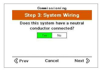
2. Select Yes if a neutral conductor is connected to the system. If a neutral conductor is connected three CTs are required to be installed.
