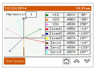
V12: Line-to-line voltage of L1 to L2.
