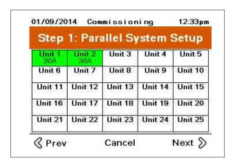
2. For parallel systems, the **Parallel System Setup** screen will be displayed. Pressing the unit ID number will cause the unit number on the screen to cycle in color default is green to orange. The LED on the front of the unit with that ID will also flash.
