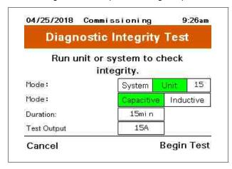
**Mode**: Select system which will cause all units in a system to operate or unit and unit ID to select a specific unit to test.
