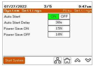
**Auto Start**: The unit shuts down when the line voltage drops below 85% of nominal. With Auto Start ON, the unit automatically returns to RUN condition when the line voltage is within 85% of nominal. The unit must be in RUN condition during the event to return to RUN condition.
