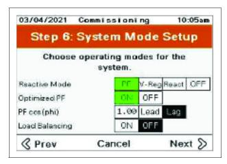
**Reactive Mode - PF**: With PF mode selected, additional parameters available for the PF mode are displayed.
