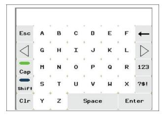
Press **Shift** icon to enable shift which will change the case of the next letter entered. A green oval indicator above the **Shift** icon indicates that the shift function is enabled.
