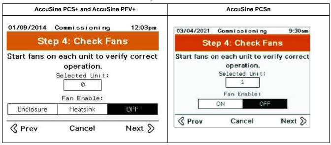
By entering the unit ID number, each fan can be operated for each unit.
