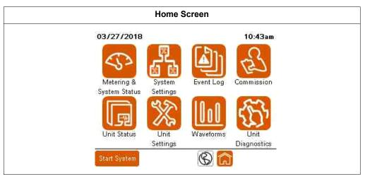
When first energized, the HMI displays the Home screen. To return to the Home screen, press the Home icon at the bottom on any of the screens. To change parameters, you must be logged in as an Admin level user. From the Home screen, you can access the following:
