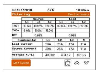
**THDi**: Total Harmonic Distortion of the current as a percentage of fundamental per phase at the Source and the Load.
