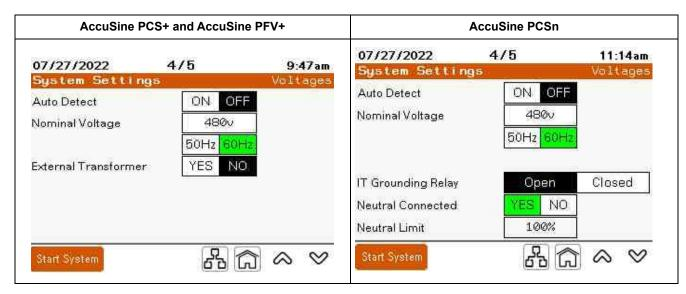
**Auto Detect**: Instructs the controller to determine nominal grid voltage and frequency when power is applied.
