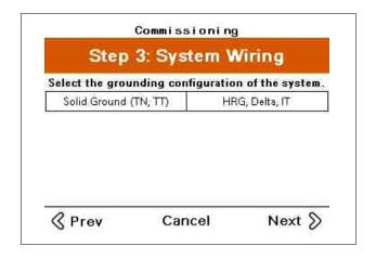
1. Select the grounding configuration of the facility where the system is installed.
