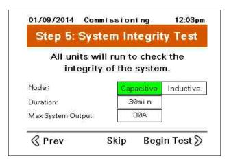
During this test, the unit will generate current in either a capacitive (Leading) or inductive (Lagging) manner. Enter the duration for the test. The test should be performed for a minimum of 15 minutes to allow the unit to reach operating temperature. Enter the maximum system output current of the system.
