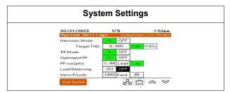
Within System Settings, you can change parameters for the system. When the unit is part of a parallel system, all of these settings for each unit must match. Changes to System Settings are synced to all units that are on-line in a parallel system.
