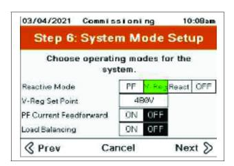
**Reactive Mode - V-Reg**: Voltage Regulation Mode. Voltage regulation mode monitors the voltage and adjusts the reactive current injected to maintain a voltage level.
