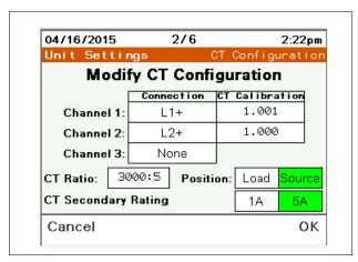
Once the unit is configured for the CTs that are installed, press **OK** to continue
