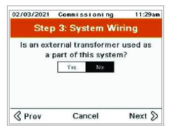
2. Change the settings on the External Transformer screen if there is an external transformer between the active harmonic filter and the voltage bus being corrected.
