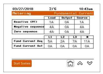
**Reactive (PF)**: Displays positive sequence reactive currents of the load, system output, and source in amperes RMS.
