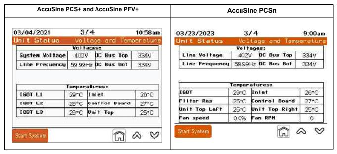
**NOTE:** The parameters of **Voltage and Temperature** screen is described below. Based on the product used, refer to the appropriate screen as required.
