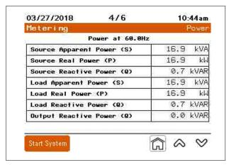
This screen displays three-phase power values of the source, load, and output of the active harmonic filter.
