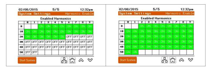
On this screen, you can select which individual harmonic orders are compensated. When ON, the harmonic order compensation is enabled. Touching any harmonic order toggles it OFF or ON.
