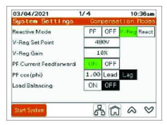
**PF Current Feedforward**: When OFF, the CTs are not required for this application. The unit maintains the V - Reg Set Point based on the terminal voltage of the unit.
