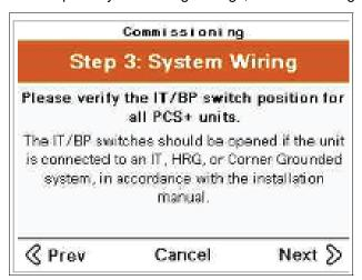
Open the IT/BP switches if the system is connected to an IT, HRG, or Corner Grounded delta system. See the Installation Manual for details on the IT/BP switches.
