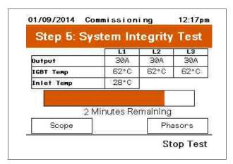
During the test, the HMI will display the output current per phase, IGBT temperature, and unit Inlet temperature. Scope and Phase allows a means to view the oscilloscope or phasor diagram of the unit during operation.
