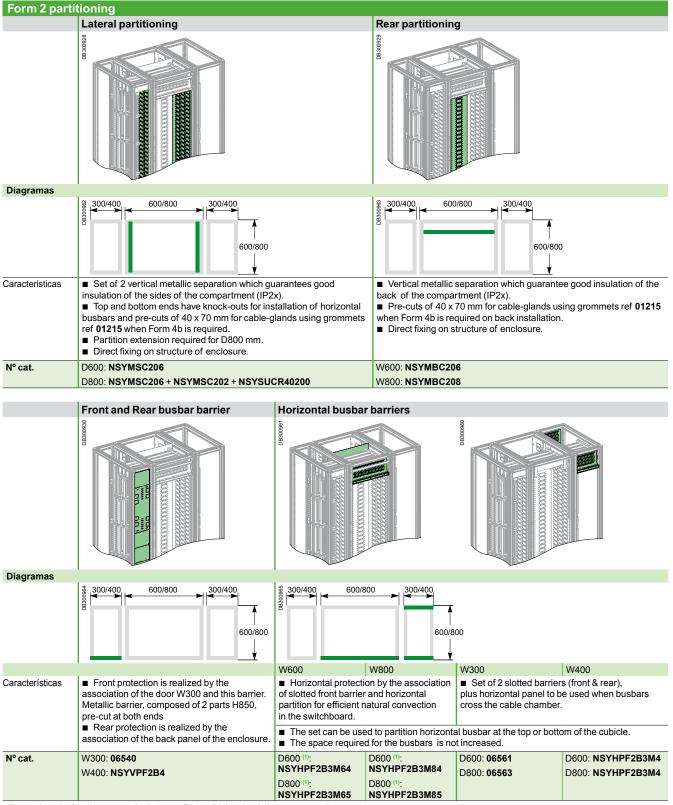
Note: when the busbars are at the bottom of the cubicle, gland plates are mandatory. (1) For an enclosure with depth of 600 mm the compartment depth is 400 mm.
