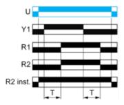
Function At: Power on Delay Relay (Summation) with Control Signal
