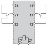
NOTE: For DC input, A1 have to be +, otherwise it would short circuit from protection module
