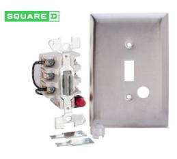
Switch, manual, 30A, 2 pole, 3 HP at 575 VAC, single phase, key operated, red 115 VAC indicator, NEMA 1 SS flush
