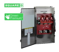
Safety switch, heavy duty, fusible, 400A, 2 poles, 250 hp, 600 VAC/DC, NEMA 4, 4X, 5, 304 steel
