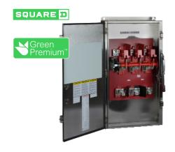
Safety switch, heavy duty, non fusible, 400A, 2 poles, 250 hp, 600 VAC/DC, NEMA 4, 4X, 5, 304 steel
