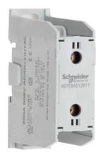
Power distribution block, Linergy, enclosed, 200A CU, 155A AL, 600 V, 1 line side lug, 1 load side lug, AL lug, panel
