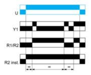
Function Tt: Retriggerable Bistable Relay with Control Signal On
