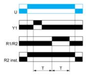
Function N: Retriggerable Interval Relay with Control Signal On
