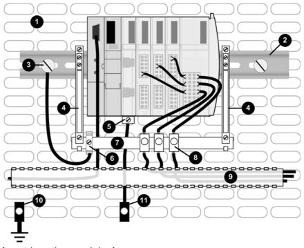
The following illustration depicts an STB island segment with an EMC kit making the analog I/O modules CE compliant.
