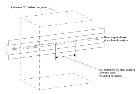
Low profile 7.5 mm (0.30 in) deep DIN mounting rail can be used with low profile mounting hardware such as flat head screws, with countersunk mounting holes.
