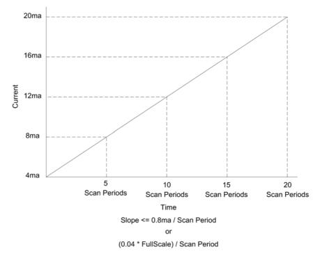
The following chart describes the relation between current and slope times for 4-20 mA current output modules:
