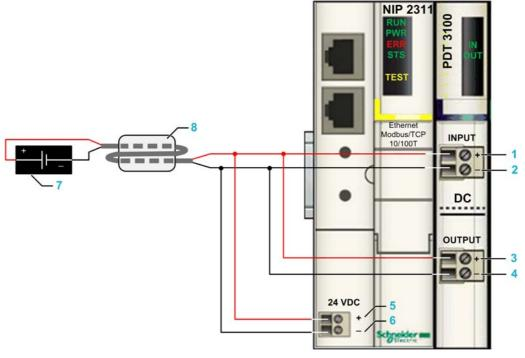
The following graphic shows you how to provide power supply wiring to the STB NIP 2311 NIM and an STB PDT 3100 standard PDM:
