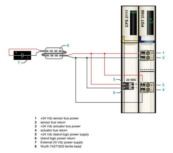
**NOTE:** To maintain CE compliance, use a Wurth 74271633 ferrite bead with NIM, PDM, BOS, and CPS power supplies. Pass the twisted pair wiring through the ferrite bead twice.
