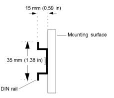
Use M5 threaded mounting hardware to affix the DIN rail to the mounting surface. Allow a maximum spacing of 150 mm (5.91 in) between each mounting hardware.
