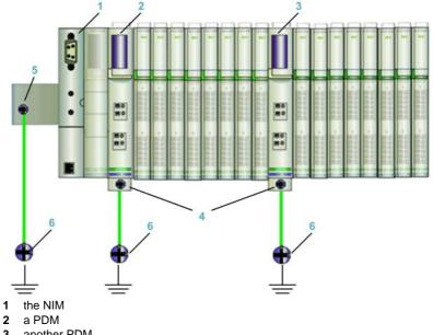
This illustration shows separate PE connections tied to PE protective ground points:
