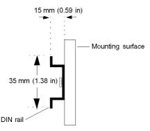
Select a DIN rail that is wider than the cumulative widths of modules you will install on it. In this example, select a DIN rail that is at least 152 mm (6 in) long.
