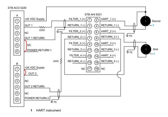
The STB ACO 0220 output module uses two six-terminal field wiring connectors. You can use either:
