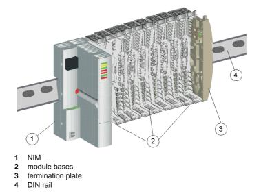
The structure of a single-segment island bus:
