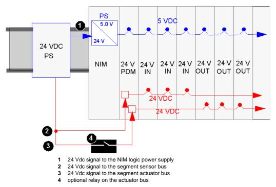
Above 130 Vac, the relay module may compromise the double insulation provided by a SELV-rated power supply.
