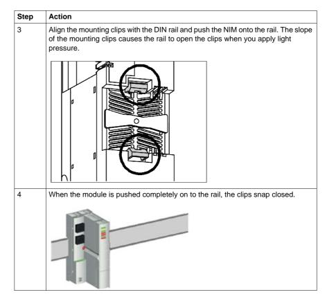
For instructions on how to remove the NIM, refer to the Advantys STB System Planning and Installation Guide.
