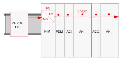
The NIM can supply maximum current of 1.2 A to the island segment modules. If your island design requires more power than the NIM can provide, you can:
