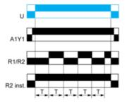
Before power-up Y1 should be permanently connected to A1. 2 timed outputs (R1/R2) or 1 timed output (R1) and 1 instantaneous output (R2 inst.)
