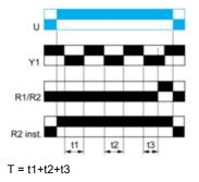
Function B : Interval Relay with Control Signal
