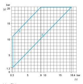
(y) Rising pressure(x) Falling pressure1: Maximum differential2: Minimum differential
