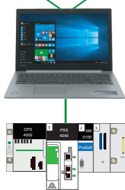
Interaction between EcoStruxure Control Expert, Prosoft Configurator for Modicon (PCM tool), and X80 PROFIBUS DP module
