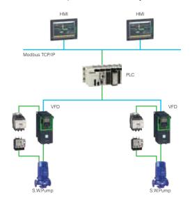
Engine Room Fans VFD Control System
