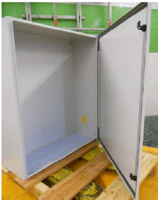
Photo 13: IPX6 test NSYCRN108300P
