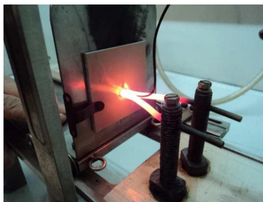
Photo 23: Glow-wire test setup (2)
