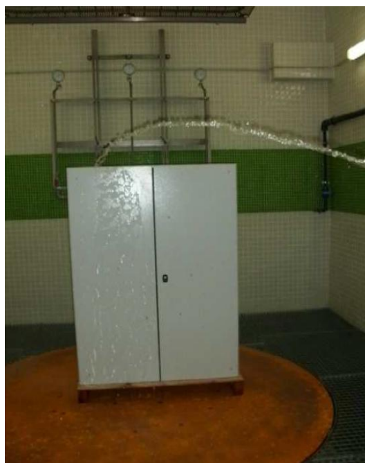
Photo 18: IPX5 test NSYCRNG1410300D
