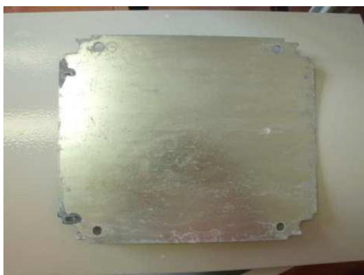
Photo 40: Mounting plate NSYMM... / NSYPMM... (severity A)
