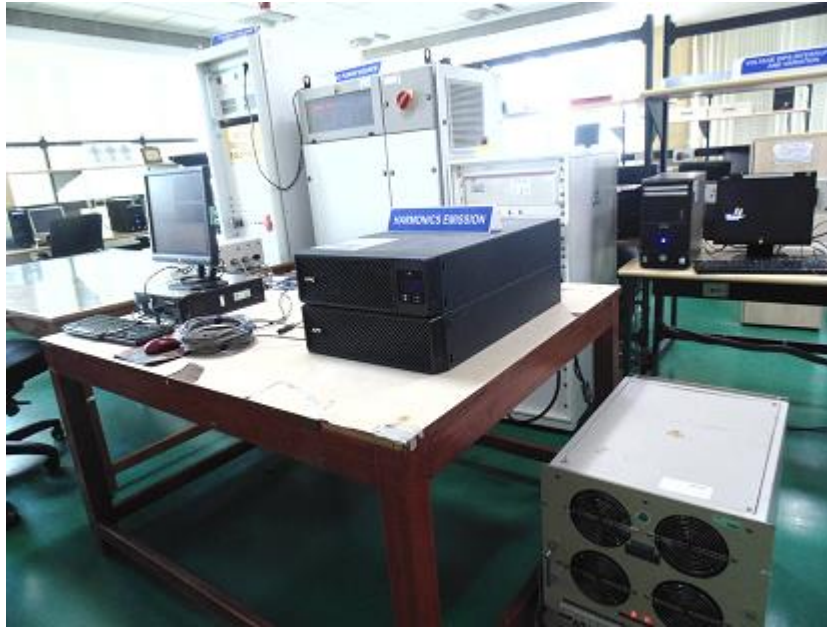
Figure 10: Photo of Harmonics current emission test setup
