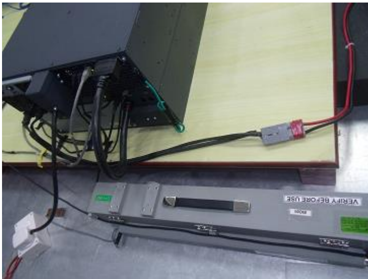
Continuous Conducted Radio-Frequency on Micro link serial communication
