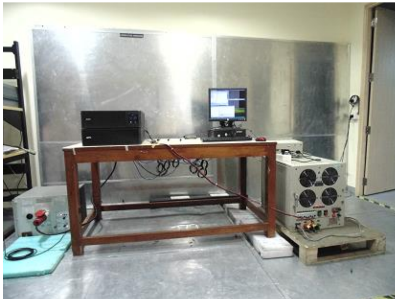
Conducted Emission Measurement: AC Input power Lines (Battery Mode)
