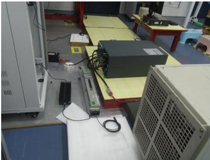
Continuous Conducted Radio-Frequency on Universal I/O 1 on NMC
