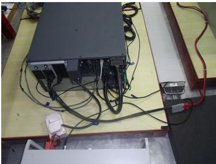
EFT on Micro link serial communication
