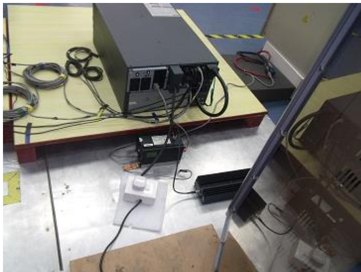
Continuous Conducted Radio-Frequency on AC output power lines
