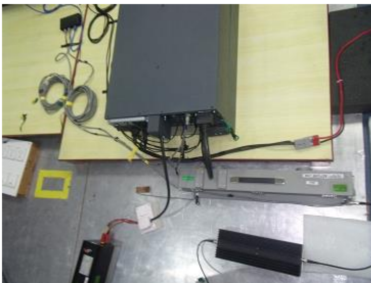
Continuous Conducted Radio-Frequency on Ethernet on Mini-rohdes
