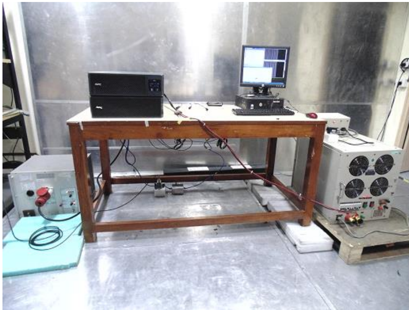
Conducted Emission Measurement: Ethernet on NMC
