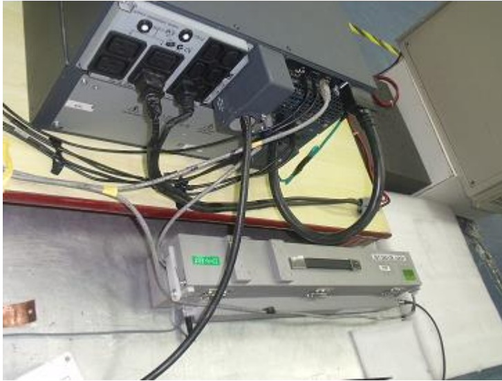
Continuous Conducted Radio-Frequency on Ethernet on NMC
