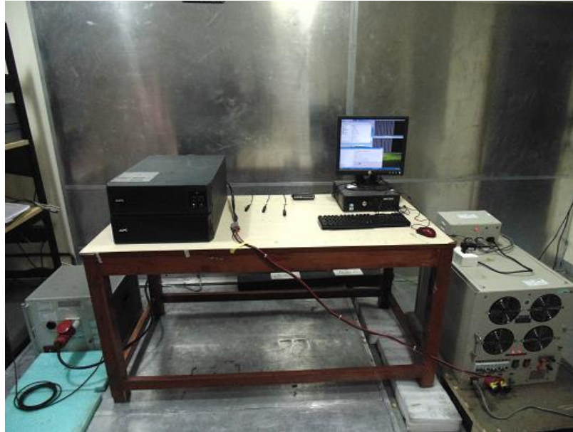
Conducted Emission Measurement: AC Input power Lines (On Line Mode)
