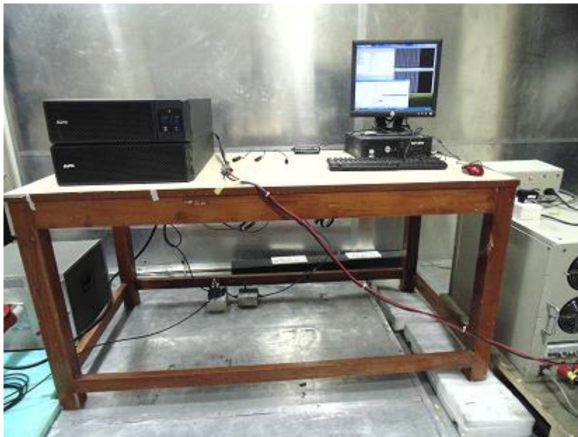
Conducted Emission Measurement: Ethernet on Mini-rohdes
