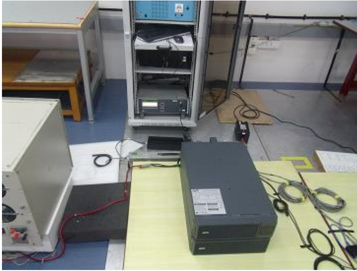
Continuous Conducted Radio-Frequency on Universal I/O on Mini-rohdes
