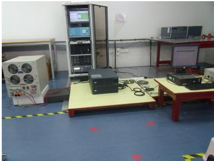
Continuous Conducted Radio-Frequency on AC input power lines
