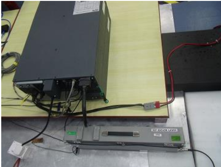
Continuous Conducted Radio-Frequency on USB
