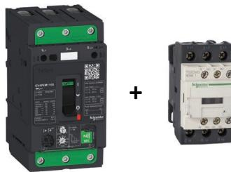
The TeSys GV4PB Motor Protection Circuit Breaker combines the functionality of a circuit breaker and an overload relay in a single device. Approved to UL 489, the TeSys GV4PB is suitable for use as a branch short-circuit protection device, and can be paired with any contactor to build a complete branch circuit for a motor load.
