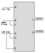
With External Device Monitoring (EDM) feedback loop
