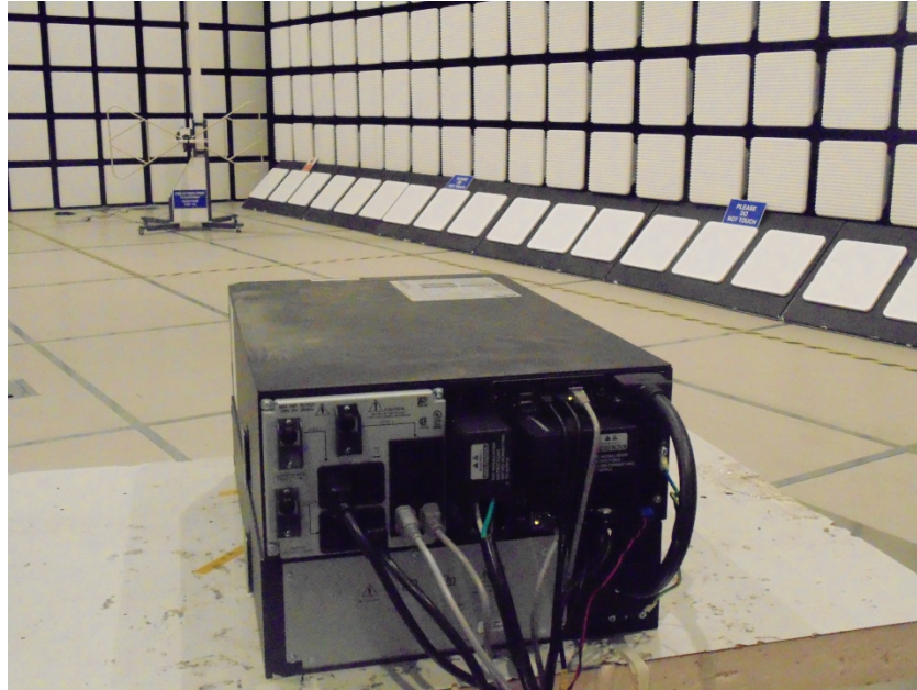
Figure 19: Radiated Emission test setup
