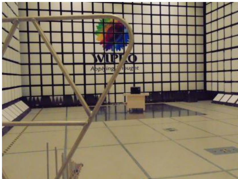
Figure 21: Radiated Emission test setup in Vertical polarization
