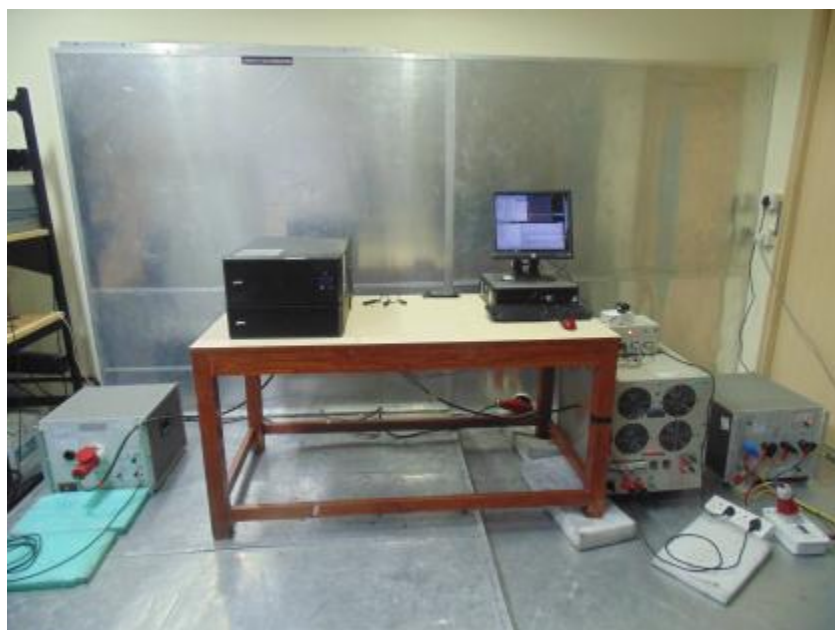
Figure 22: Conducted Emission test setup
