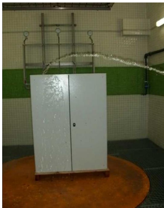
Photo 18: IPX5 test NSYCRNG1410300D
