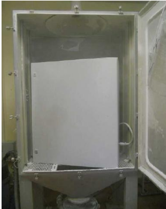
Photo 11: IP6X test NSYCRN108300P (1)
