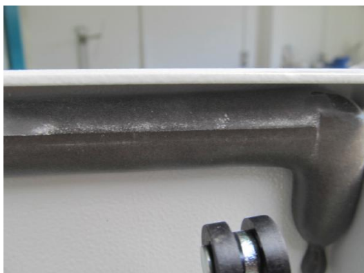
Photo 17: IP5X test NSYCRNG1410300D
