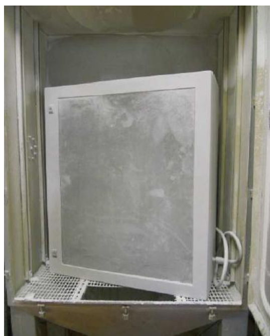
Photo 14: IP6X test NSYCRN108300T (1)
