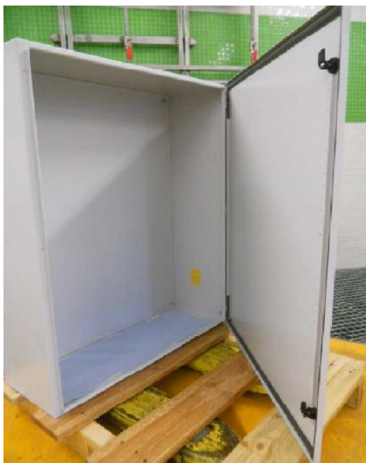
Photo 13: IPX6 test NSYCRN108300P
