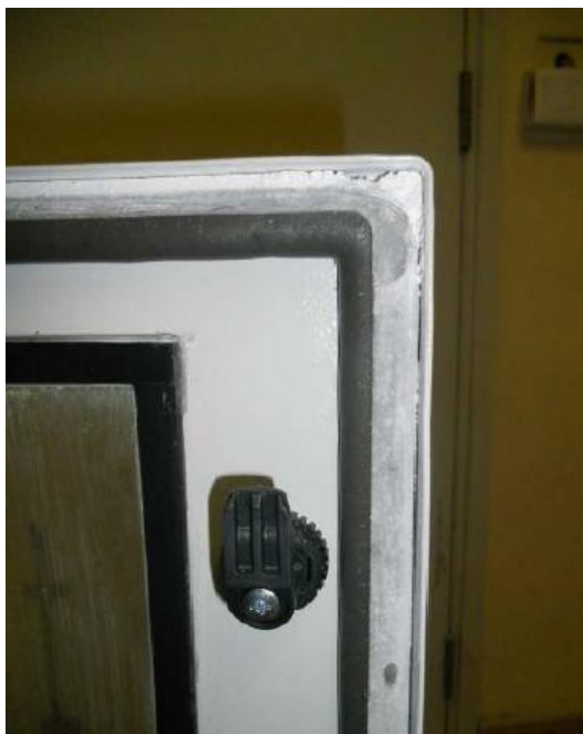
Photo 15: IP6X test NSYCRN108300T (2)
