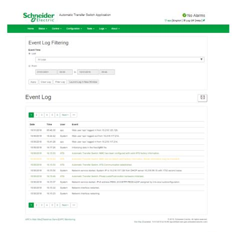
To open the log in a text file or to save the log to a disk, click on the floppy disk  $\square$  on the same line as the **Event Log** heading.
