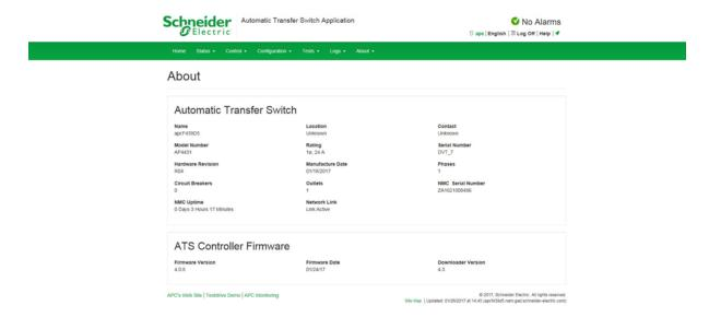
The hardware information is useful to APC by Schneider Electric Customer Support for troubleshooting problems with the ATS. The serial number and MAC address are also available on the ATS itself.
