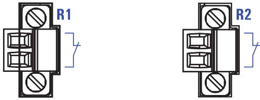
Figure 3: Pin assignment of the signal contact
