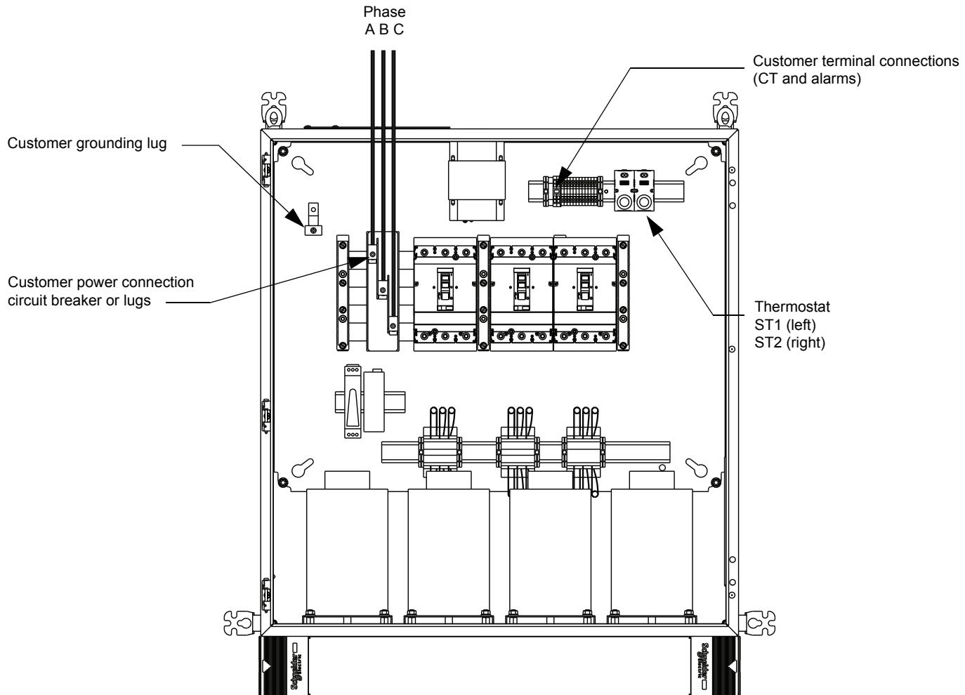
**NOTE:** A capacitor bank is a load. The only power cabling to be done is the incoming cable to the line side of the incoming breaker or incoming lugs.
