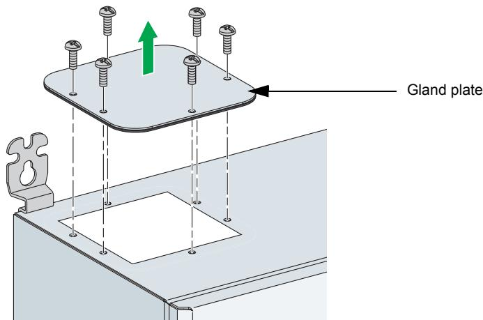
2. Use drills or punches (depending on the diameters of the holes to be made) to allow the routing of:
