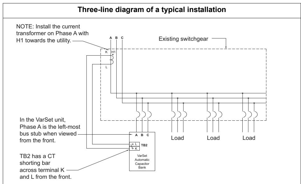
The CT should be installed with the correct polarity.
