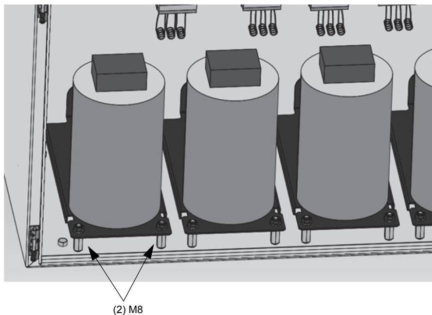
6. Carefully lift the capacitor plate out from the bank. Avoid scratching or damaging other components when removing. The maximum weight of two capacitors and the plate is 25 lbs (11.34 kg).
