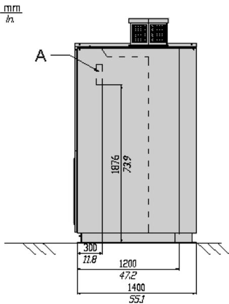
A Outlet Terminal, Control Circuit
