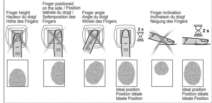
**en** Storage capacity: 200 users with up to 2 fingerprints. Recommendations to ensure optimum fingerprint recognition:
