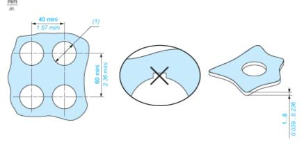
(1) Ø30.75 mm recommended (Ø30.5 mm  $_0$  +0.5) / Ø1.21 in. recommended (Ø1.20 in.  $_0$  +0.019)
