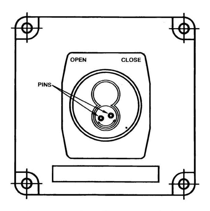
To remove cover when combinated core is not in place: remove cover screws, insert screwdriver between pins, rotate locking mechanism either clockwise or counterclockwise, slide cover down and lift off.
