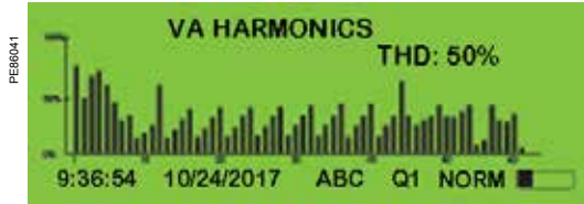
PowerLogic ION8650 front panel harmonic display.
