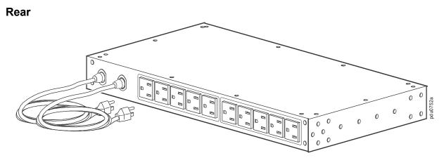
**Input power cords:** The two cords connect the ATS to two separate power sources (A, B). The switch draws power from the preferred source and automatically switches to the secondary source when necessary. The two (2) 2.44-m (8-ft) power cords have NEMA 5-15P plugs.
