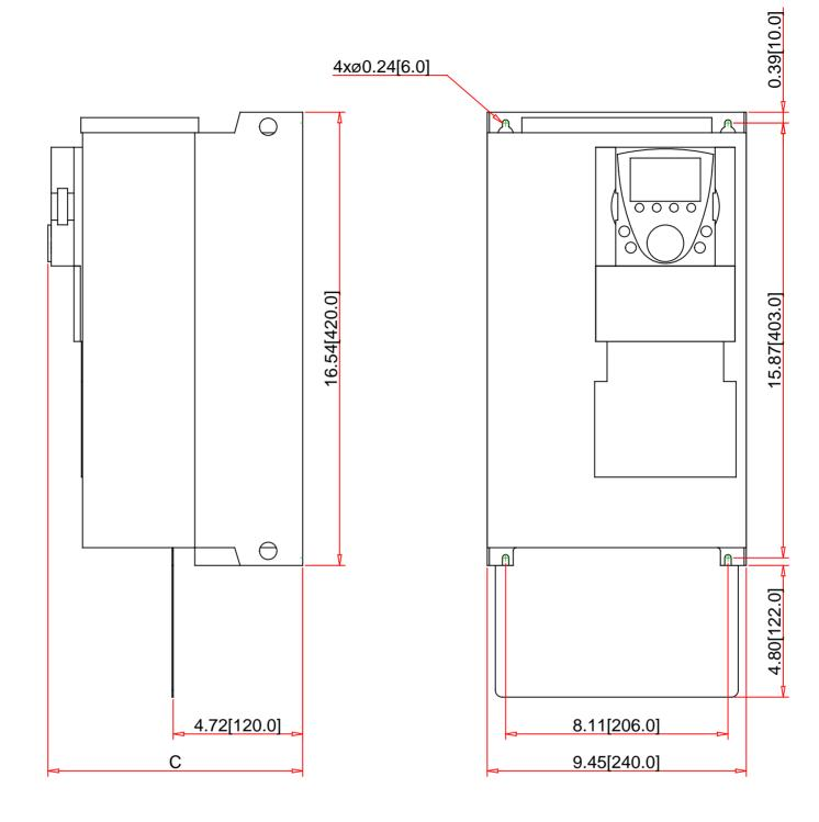
Optional EMC grounding plate is shown, it may be removed if not needed in the application.
