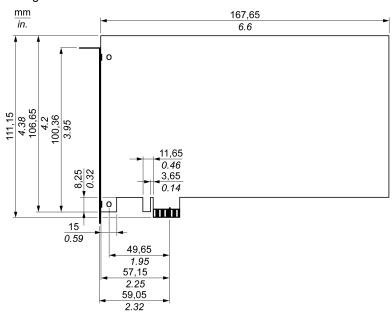
The figure shows the dimensions of the standard half-size PCle card:
