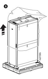
**NOTE:** System integrators stop the unpacking process at Step 8. Install your equipment, then follow the Repacking Instructions on side 2 of this sheet.
