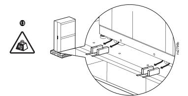
Attach the ramp (AR9000RAMP, not provided) to the pallet near the rear of the cabinet. See the ramp documentation for instructions.
