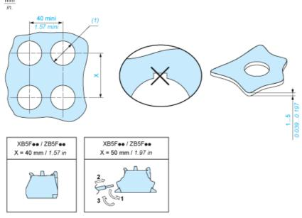
(1) Ø30.75 mm recommended (Ø30.5 mm  $_0$   $^{+0.5}$ ) / Ø1.21 in. recommended (Ø1.20 in.  $_0$   $^{+0.019}$ )
