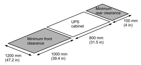
The UPS system requires a minimum rear clearance of 100 mm (4 in). There is no side clearance required for installation.
