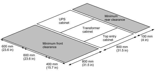
The UPS system requires a minimum rear clearance of 100 mm (4 in). There is no side clearance required for installation.
