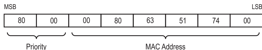
Figure 8: Bridge Identifier, Example (values in hexadecimal notation)
