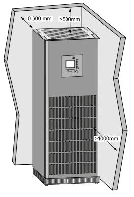
**NOTE:** The clearance dimensions given above are published for airflow and service access only. Consult with the local safety codes and standards for additional requirements in your local area.
