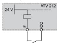
“PLC” position with PLC transistor outputs
