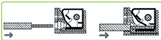
Push and stay spring clamp terminal: insert without tool
