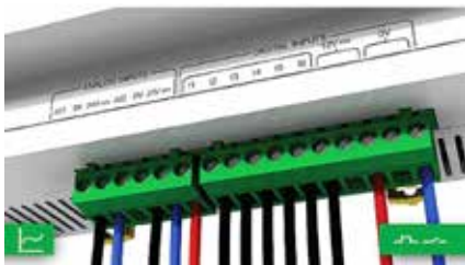
Power supply to analogue and digital inputs
