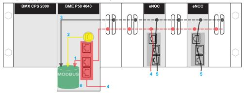
**red:** These requests are sent to the IP address of the CPU. **vellow:** These requests are from the USB port of the CPU.
