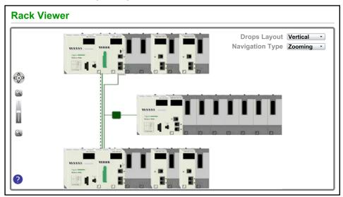
The Hot Standby connection (dashed line) is green when the Hot Standby link is healthy.
