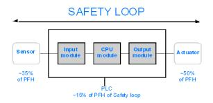
For the calculation of the PFD/PFH values of an example system, a maximum of 15% is assumed for the PLC. For the PFD/PFH values of the Quantum Safety modules, see *Available Safety Products*, page 17.
