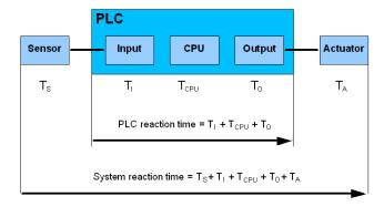
The system reaction time must be less than the process Safety time.
