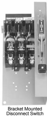
The 9422 Bracket Mount Disconnect Switch is designed for combiner boxes and control panel applications. The Bracket Mount Disconnect Switch is shipped with the switch and external handle assembled to a bracket, ready for quick installation. A protective trim plate is provided to prevent any mounting screws from being accessible from the front. The trim plate also provides an attractive installation feature. The switches are fully compatible with the 9423 closing mechanisms.
