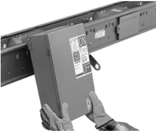
Plug-in units are positioned along the busway length by notches in the busway housing top that accept the mounting hooks of the plug-in unit. This aligns the plug-in unit connectors with the plug-in opening. After the unit is positioned on the busway it is allowed to swing down into the plug-in opening where the connectors make contact with the bus bars. This is accomplished in a “hook-swing” sequence of motions.
