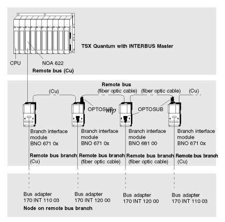
The conversion from copper cable to fiber optic cable is done with OPTOSUB or OPTOSUB PLUS, depending on the module used (see section *Transition from Copper Cable*  $\leftrightarrow$  *Fiber Optic Cable*, page 14).
